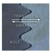
Thread flanks can slide. Nut can move relative to bolt.
