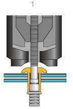
Insert the fastener into the hole and slip the installation tool over the pintail.
