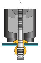
continued pulling on the pintail expands the sleeve to maximum allowable diameter. As the shear ring reaches the backside of the work piece it breaks and catches on the tapered annular grooves, keeping high pressure on the blind side of the work pieces as the pin continues to draw down inside the sleeve.
