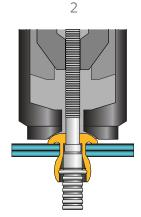
Press the trigger to initiate pulling action. As the tool pulls on the pintail, the shear ring feature on the pin pulls inside the sleeve fully expanding the diameter and drawing the work pieces together.
