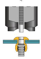
A solid circle lock between the pin and sleeve is formed just prior to the pin breaking flush with the sleeve head, completing the installation.
