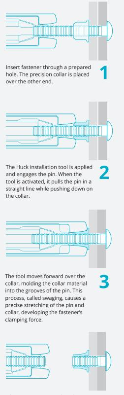
When swaging is complete the pintail is automatically tensioned off, flush with the end of the collar. The tool then pushes off from the collar. The result is a permanent, mechanically locked fastener
