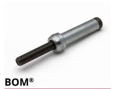
Blind, Oversize, Mechanically locked fasteners. Unique push-and-pull installation design for ultimate locking strength from blind-side install.
