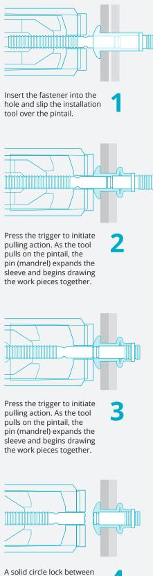
A solid circle lock between the pin and sleeve is formed just prior to the pin breaking flush with the sleeve head, completing the installation.
