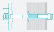
The pin is then separated in tension at the break neck groove.
