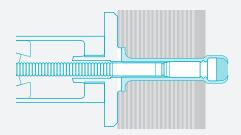
Continued pulling on the pintail forms a mechanical lock between the pin and sleeve end. The anvil on the installation tool then countersinks the fastener head into the top of the material to a preset depth set by the anvil. The anvil's large bearing face then prevents further travel of the sleeve head into the top material.
