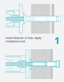
The Huck installation tool is placed over the pintail. When the trigger is pressed, the nose assembly jaws pull on the pintail, drawing the pin though the sleeve, causing the blind side sleeve to expand, partially setting the sleeve in the top sheet and pulling out all the sheet gap.
