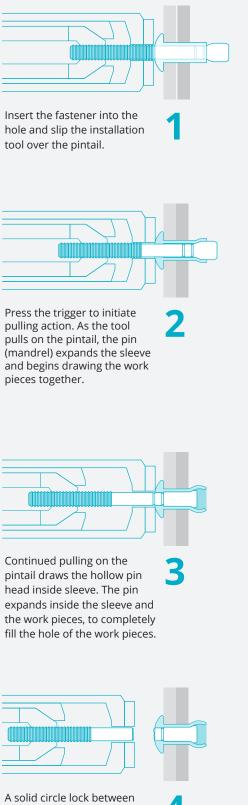
the pin and sleeve is formed just prior to the pin breaking flush with the sleeve head, completing the installation.
